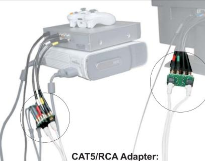
A single or dual CAT5 cable extends AV components, HD TV and Digital Audio up to 50 feet. (Impedance matching required for distances over 50 feet)
